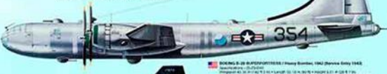
BOEING B-29 SUPERFORTRESS / Heavy Bomber, 1945 Wingspan: 42 m (137 ft 9 in) • Length: 36.6 m (120 ft 1 in) Height: 15.2 m (49 ft 9 in) • Max Speed: 580 km/h (360 mph)
