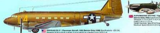
DOUGLAS DC-3 / Passenger Aircraft, 1935 Wingspan: 28 m (92 ft) • Length: 29.7 m (97 ft 6 in) Height: 9.7 m (31 ft 8 in) • Max Speed: 336 km/h (209 mph) First Flight: December 17, 1935
